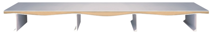
SPS - the existing worn/corroded plate and new top plate are bonded together with a solid elastomer core forming a fully composite structure.
